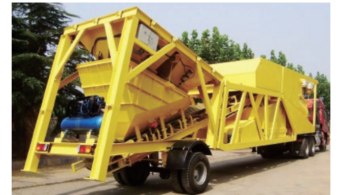
● Mobile concrete batching plant is being transported
