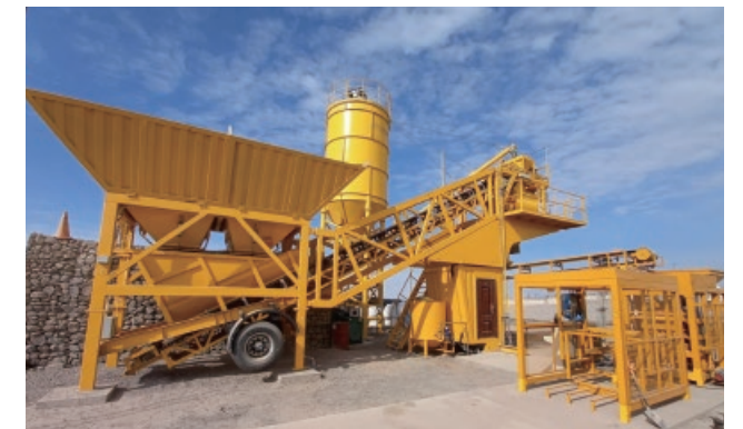
● Mobile concrete batching plant is working
