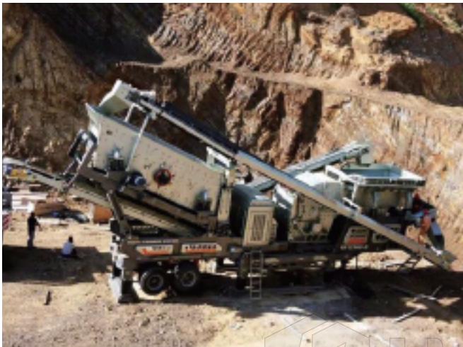
◀ Mobile impact crusher and screen
